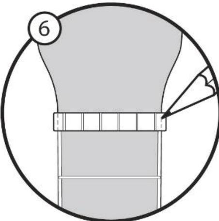
6. Once you've got the thickness and height correct, you just need to sand the ends of the nut so that they are flush with the neck. Graph Tech adds a little "meat" on the ends of their nuts, so you will always end up with a nice, flush finish. Just use a pencil and mark the ends of the nut that are sticking out, remove it from the neck and sand it to your marks.
