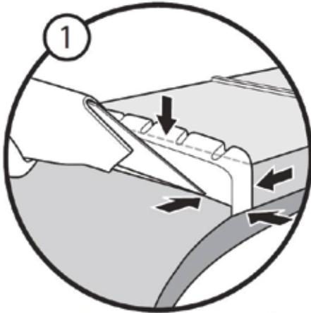
1. Remove the strings. Trace around (score) every edge of the nut with an exacto knife to prevent the lacquer from sticking to the nut before you remove it.
