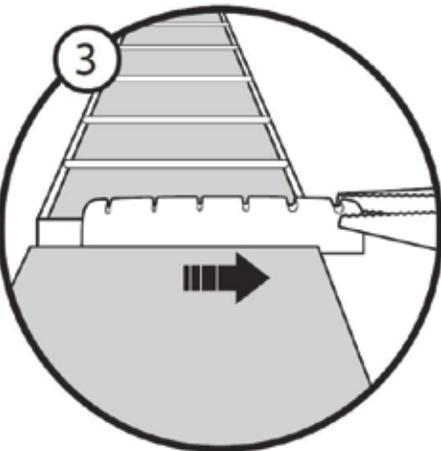
3. When it is sticking out the side, pull it out in the same direction with a pair of pliers, like you'd pull out a tooth. Scrape or file the nut slot free from old glue and finish residue while making sure that the slot remains square.
