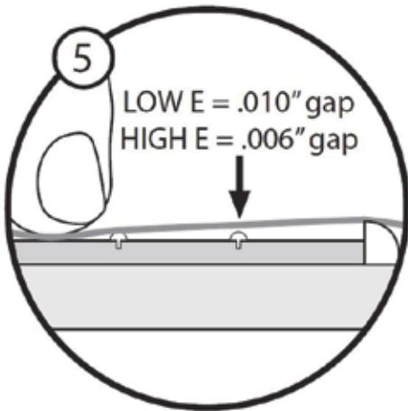
5. Restring the high and low E strings and tune to pitch to check for the correct height. For Electric Guitars, Push down on the third note of the low E string you are looking for a .010" gap between the low E string and the first fret and a gap of .006" on the high E string.
