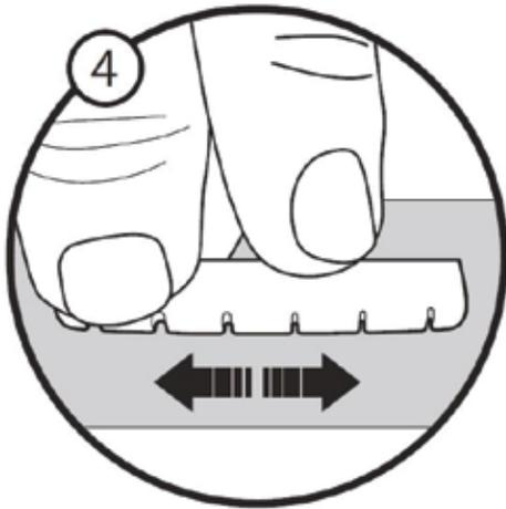
4. See if your new Graph Tech nut fits into the slot without force. If it's too thick, place a 400 to 600 grit sand paper face up on a flat surface and sand down the side of the nut until it fits in the slot snugly, but is easily removable.
