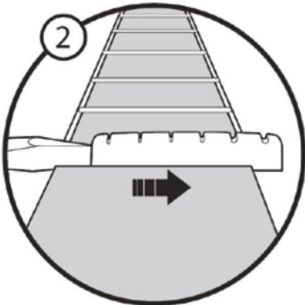
2. If the nut is not sitting in a slot, and just butted up against the neck, usually a light tap with a small block will set it free. If it is sitting in a slot, gently tap it out sideways using a hammer and a screwdriver. If you pull it out upwards, you risk taking some of the wood with it.
