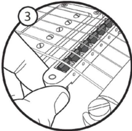
3. Now install strings and tune your guitar to concert pitch. Adjust the string height by turning the thumb wheels on the bridge posts. Raise or lower the treble and bass sides of the bridge until correct string height (measured in Step 1) is achieved.
